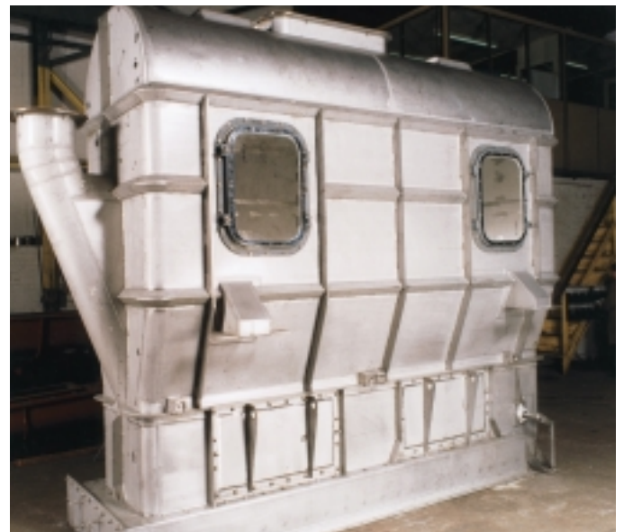
Fluid bed cooler for sugar incorporating cooling tubes
