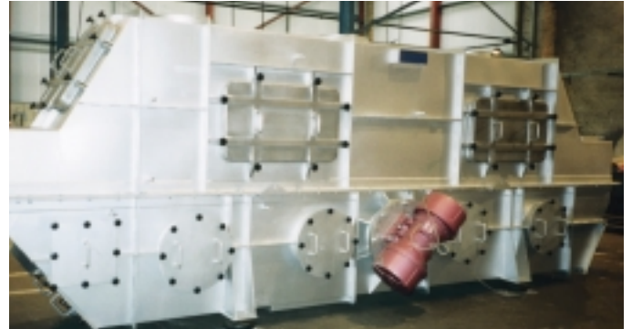
Vibrating fluid bed dryer for cooked grains
