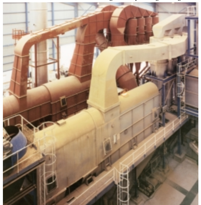
Two fluid bed dryer/coolers for sand
